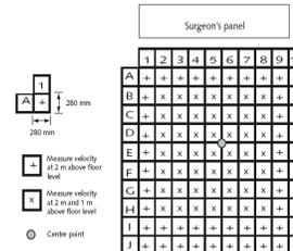
(Diagram from guidance – misprint in column 2 – the “x”s should be “+”s)
